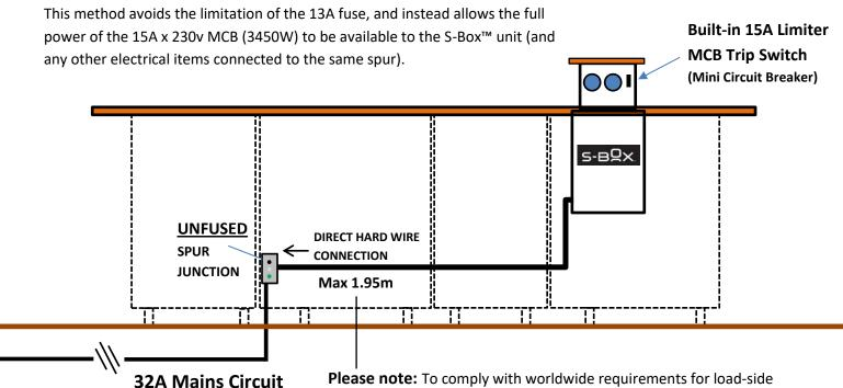
Please note: To comply with worldwide requirements for load-side protection and change of cable core size (32A 2.5mm2 building wiring changing to 1.5mm2 SBOX cable) the cable length from the S-BOX™ to the open end of an unplugged cable (Option 2), must be less than 2 metres.
